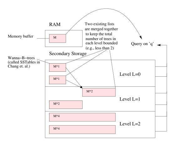
Figure 3.3: Basic LSM-tree Design
