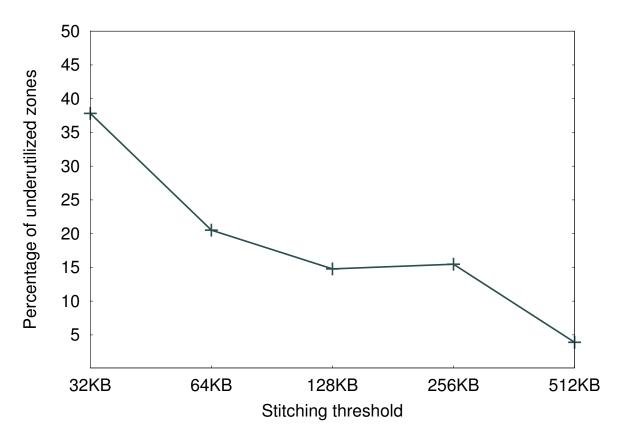
Figure 4.9: Percentage of under-utilized zones (< 75%) with different stitching thresholds after inserting 34GB of data in KVFS
