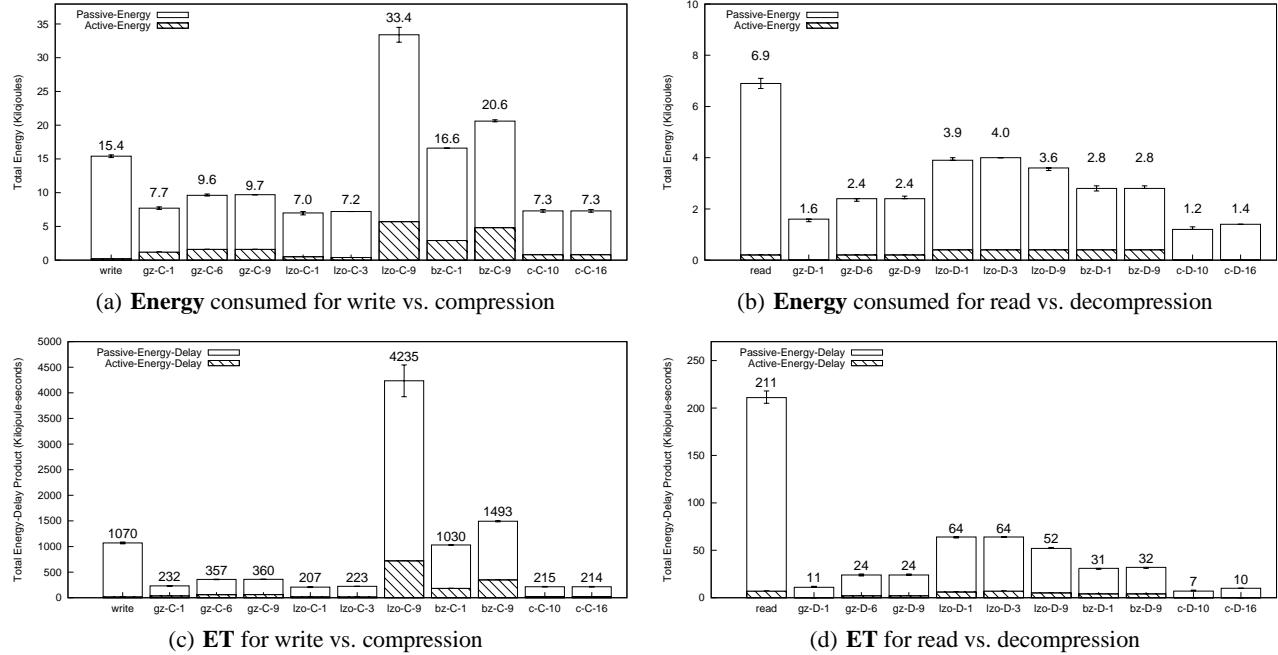
**Figure 6: Zero file: The energy and energy-delay product (ET) for compress-write/decompress-read a 2GB zero file.**
