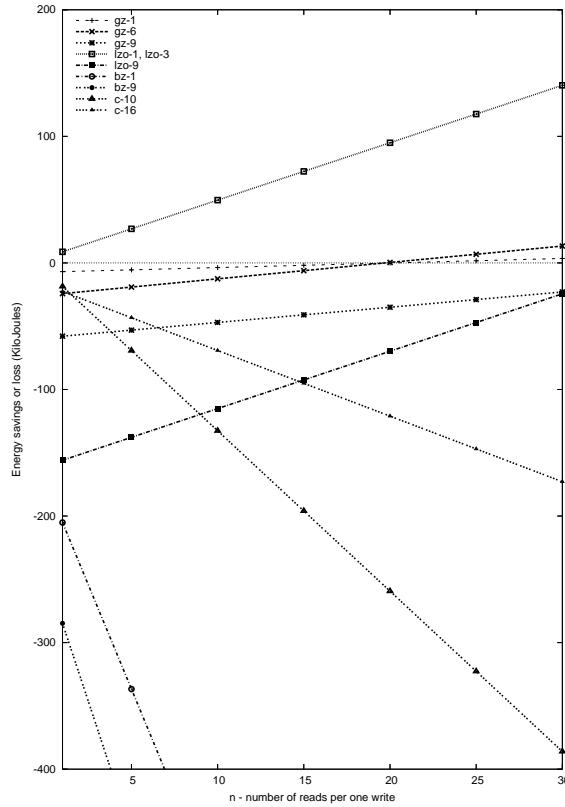
**Figure 3: Energy savings or loss ( $E_{sav}$ ) compared to plain read and write as a function of the number of reads per one write for text files on the server system. The lzo-1 and lzo-3 results are so close, that we put them on the same line.**
