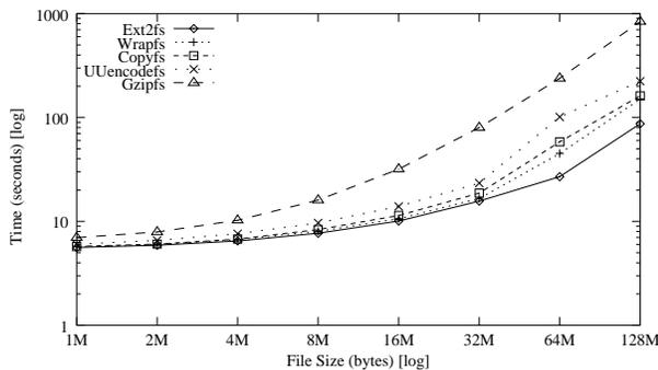
Figure 6: The Bonnie benchmark performs many repeated reads and writes on one file, as well as numerous random seeks and writes in three concurrent processes.
